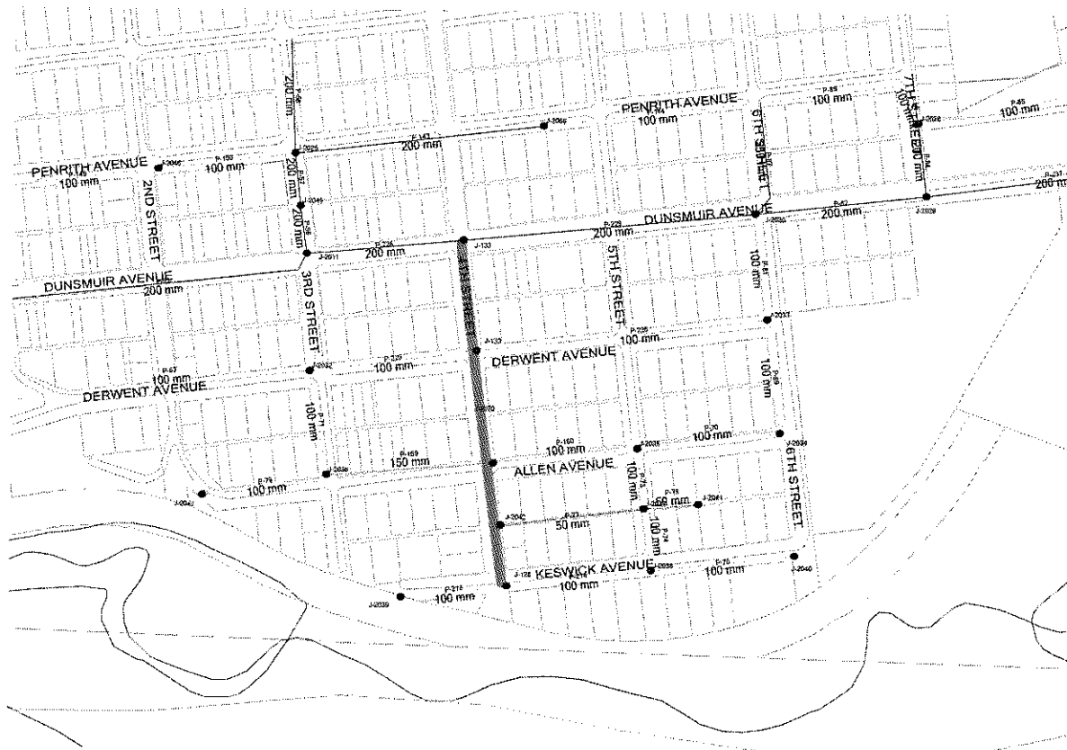
Figure 6.3.2 – New pipe on 4 th Street
