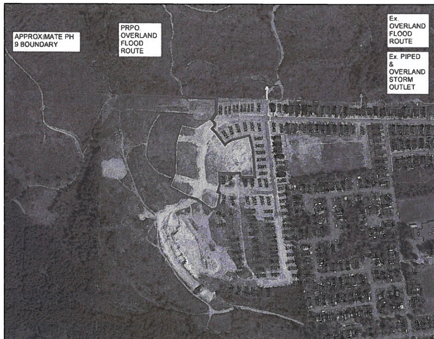
Figure 1: Approximate Phase 9 boundary and stormwater outfall locations. (image provided by McElhanney Consulting Services Ltd.)
