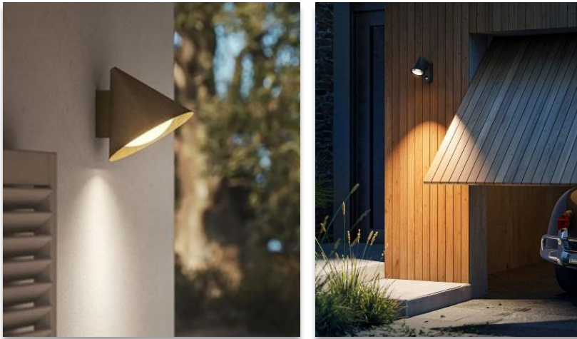
Figure 11.6-13: Example of shielded directional lights (guideline 5d)
