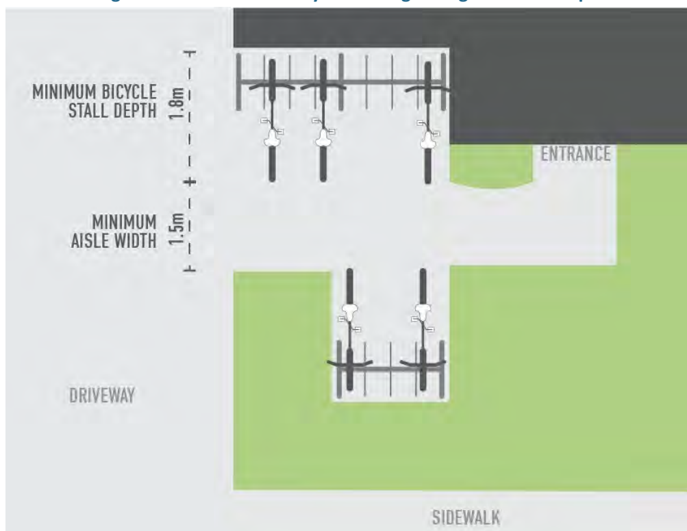
Figure 9-4. Short-Term Bicycle Parking Configuration Example
