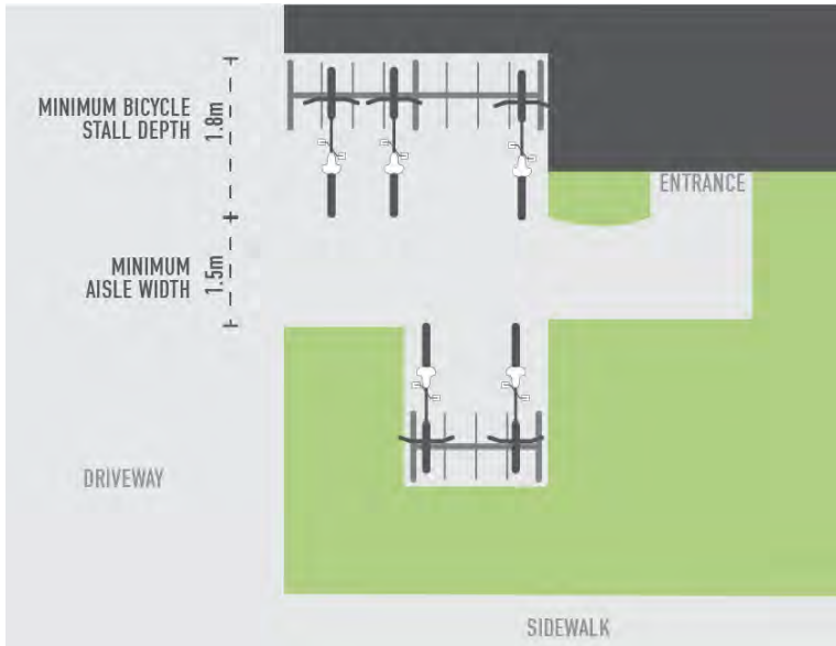
Figure 9-4. Short-Term Bicycle Parking Configuration Example
